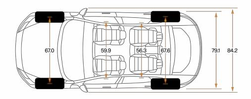
Dimensions (mm): L-4840 mm H-1534 mm W-2139 mm Wheelbase (mm): 2999 mm Tyre specs: 21" 265/45 295/40 – 22" 265/40 295/35 Luggage volumes front/rear (liters): 15 L/526 L
